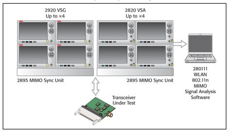
The System-2800 and System-2900 can be configured into high-performance two-, three-, or four-channel systems to test WiFi, WiMAX, and other MIMO devices and equipment.
