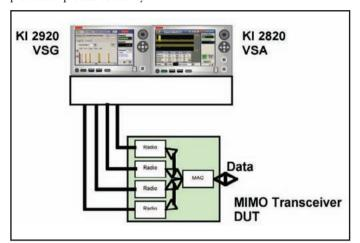
The Models 2820 and 2920 are used in a SISO configuration with a switch multiplexer to test the individual transceiver radios of MIMO devices in production applications.
