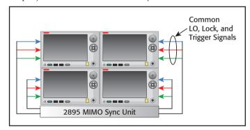
Precise and stable synchronization is achieved by providing common LO, common clock, and precise trigger signals to all of the signal analyzer or signal generator instruments.
